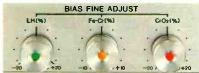
Bias Fine Adjustment allows precise fine tuning for optimum response.
