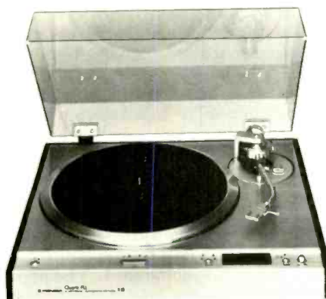
Pioneer PL-610 with quartz lock and direct drive
