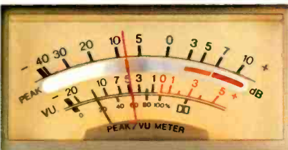
AIWA's exclusive Double Needle Meters let you check both VU and Peak levels at a glance because they're combined on the same meter.
