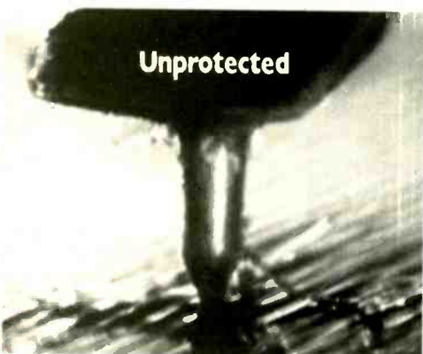
Magnification shows the record vinyl wearing away.
