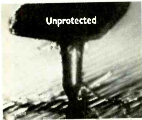
Magnification shows the record vinyl wearing away.
