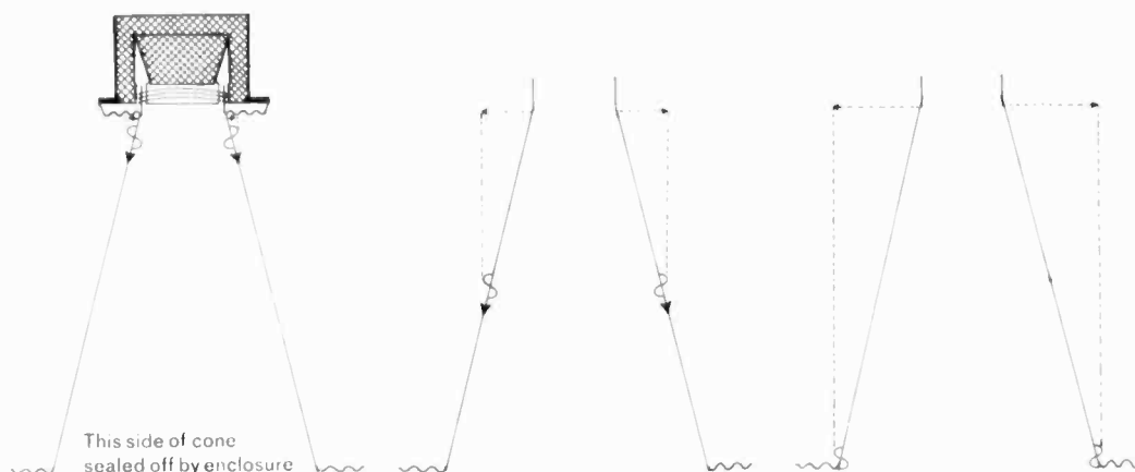
Diagram from Ohm Acoustics indicates how Walsh driver works. Conventional magnet-and-coil driver (top) produces wave in cone, which in turn excites air in contact with it. As wave moves down cone (second and third diagrams) it stays synchronized with acoustic wavefront (dotted vertical lines), progressively reinforcing it.
