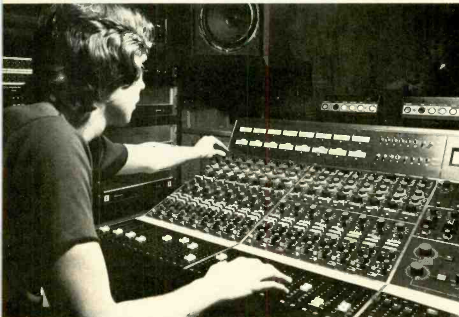
Student engineer Michael Barry prepares the console for the first take. The meters at the top of the console indicate what's happening at each microphone location in the studio. The sixteen rows of knobs, switches, and faders allow the engineer great flexibility in signal processing, routing, and balancing of each microphone output. Later on, these same controls may be used to mix down the completed multitrack tape.
