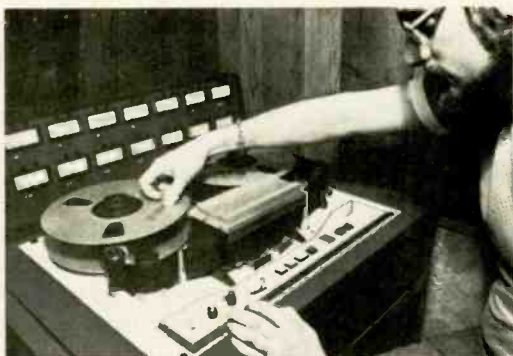
The Big Apple's sixteen-track tape recorder is readied for the day's recording activity. Note the size of the splicing block just below technician Marc Paley's arm.
