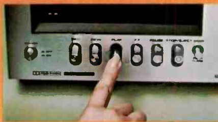
Switch from one mode to another, bypassing the Stop lever.
