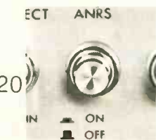
Automatic Noise Reduction System for improved signal-to-noise ratio.
