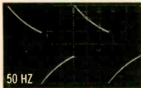
Square-wave response. Upper 50-Hz photo made in "normal" mode, lower one in "test."
