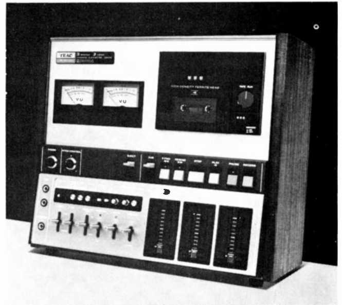
Only a few models are following up on last year's big-news feature—the separate playback or monitor head. This is the 1975 version of the $1,000 Teac 850, visibly changed in a number of ways from the prototype displayed a year ago. Lower part of control panel includes Dolby calibration controls, which are inaccessible or difficult of access to user in many models as hedge against unintentional misadjustment. When correctly used, however, controls allow tailoring of Dolby action to tape type.
