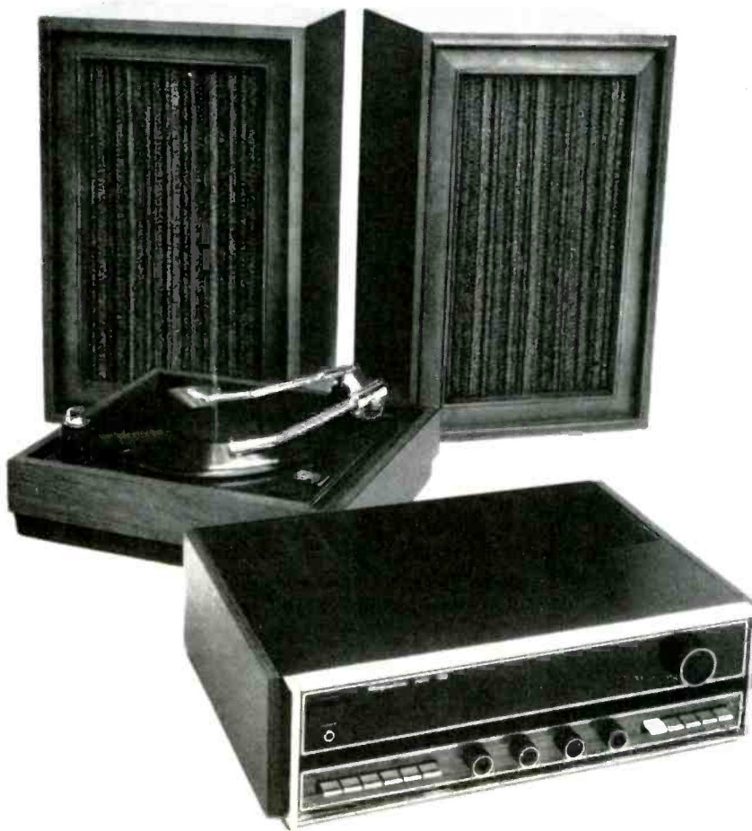
The Ultimate Magnavox (Model 9299)—Solid-state Stereo FM/AM Radio-Phonograph. 150 watts IHF music power. Air-suspension speakers (two 12" bass woofers, two 1000 Hz. exponential horns). Record player has synchronous 4-pole motor, damped cue control, magnetic cartridge, adjustable stylus pressure, muting switch.
