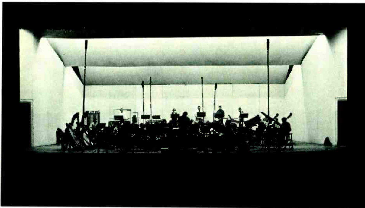
The microphone setup at the Eastman Theater during a recent recording session illustrates one method of capturing four-channel sound. The four microphones in the center pick up the group much as they might for conventional stereo, with two mikes on each channel to broaden the coverage. The nearer mikes at the sides are aimed away from the musicians to pick up reverberation from the auditorium. The music being taped is Warren Benson's Symphony for Drums and Wind Orchestra with the composer directing the Eastman Wind Ensemble.
