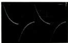
Response to 50-Hz square wave.
