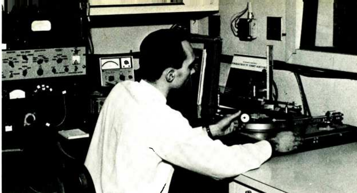
The author checks stylus force, standard preliminary to any turntable test. Signal from test record is fed through equalizer (light panel) to instrumentation that measures speed irregularities from pitch changes.
