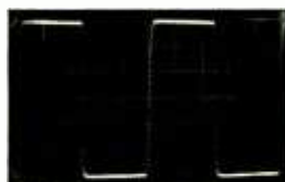
Response to 10-kHz square wave.
