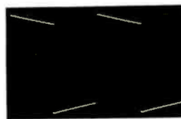
Square-wave response to 50 Hz, left, and to 10 kHz.
