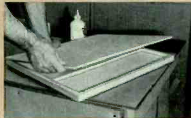
1. Cabinet back cover being assembled. Heavy plywood walls are further strengthened by thick wood braces, forming a strong, rigid panel with cavities.
