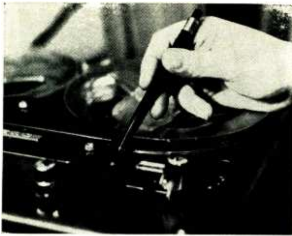
A recommended place to mark a tape for editing or splicing is just where it emerges from head-cover.
