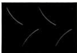
Square-wave response to 50 Hz, left, and to 10 kHz.
