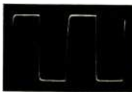
Square-wave response to 50 Hz, left, and to 10 kHz.
