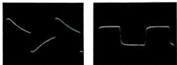
Square-wave response to 50 Hz, left, and to 10 kHz.
