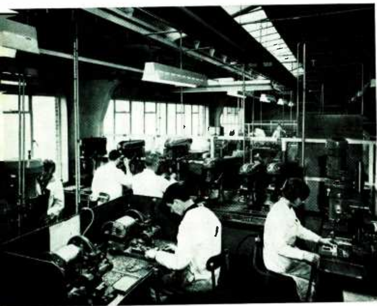
Fabricating tone arm counterweights at SME Ltd.
