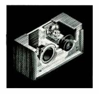
Cutaway view shows components and L/C network in a sophisticated glass fibre damped acoustic enclosure.
