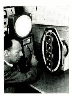
Strobe tests cone movement at EMI.
