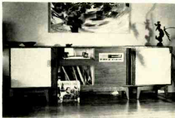
The Swedish Modern cabinetry housing the system at right has tambour doors which can be drawn across to conceal the Garrard 98 changer and Sargent-Rayment SR-380 FM/AM stereo tuner. The Sargent-Rayment dual 20-watt amplifier is housed behind the blank panel below the tuner. The speakers are Wharfedale WS2 systems in matching enclosures.
