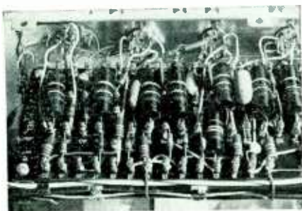
Close-up of terminal board on which most of the parts are mounted. Lugs are numbered to guide the kit builder. Note connections from the board to the tube sockets below. One board is used for each channel.
