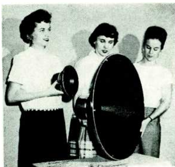
Fig. 4. David and Goliath—or Electro-Voice's 8-inch wide-range speaker seen alongside its tremendous 30-inch woofer.
