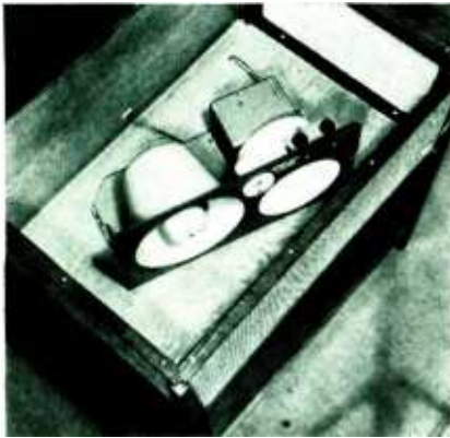
Speakers swivel for stereo directionality.
