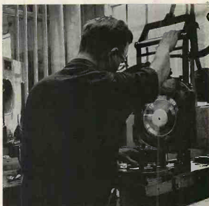
Scenes at the Philips plant. At left: minute faults found in positive "mother" matrix can be corrected with aid of engraving tool under the microscope. At right: press operator trims edges of record, inspects it visually (and sometimes aurally) and slips it into inner sleeve.
