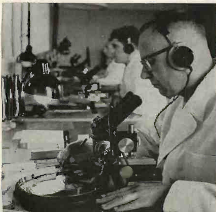
Scenes at the Philips plant. At left: minute faults found in positive "mother" matrix can be corrected with aid of engraving tool under the microscope. At right: press operator trims edges of record, inspects it visually (and sometimes aurally) and slips it into inner sleeve.
