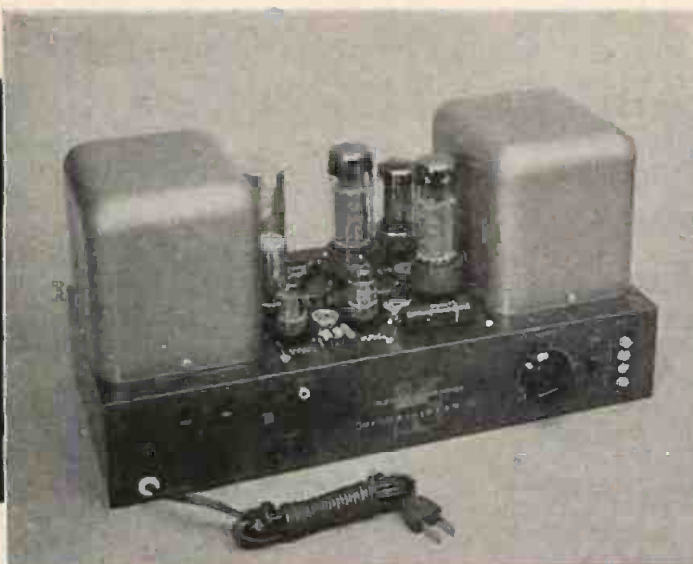
The printed-circuit board mounts on the base assembly between the output (right) and power transformers, as pictured above.
