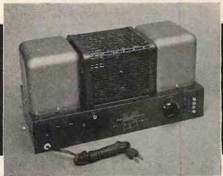
Positioning a protective metal cage over tubes is final step in U-L-II construction. Completed amplifier looks like this.
