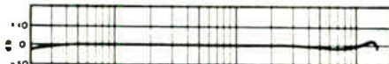
Model RG-555 Cartridge Frequency response 33½ rpm record with compensation for Decca curve.
