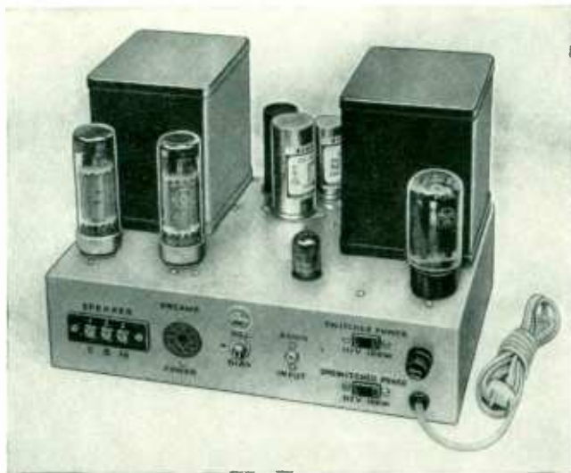
The Gray AM-50 50-watt power amplifier unit.
