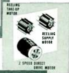
Three motors,—direct drive,—fastest forward and reverse
