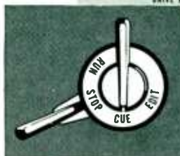
Editing and cueing, plus monitoring from tape and input while recording
