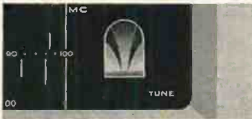
Precision-ray tuning eye makes it simple to tune precisely on both AM and FM.
