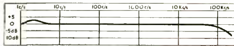
Wide-band response curve of amplifier, 2 cycles per second to 160,000 cycles per second, in comparison with the audible band 20 c.p.s. to 15,000 c.p.s., assures effective feedback.
