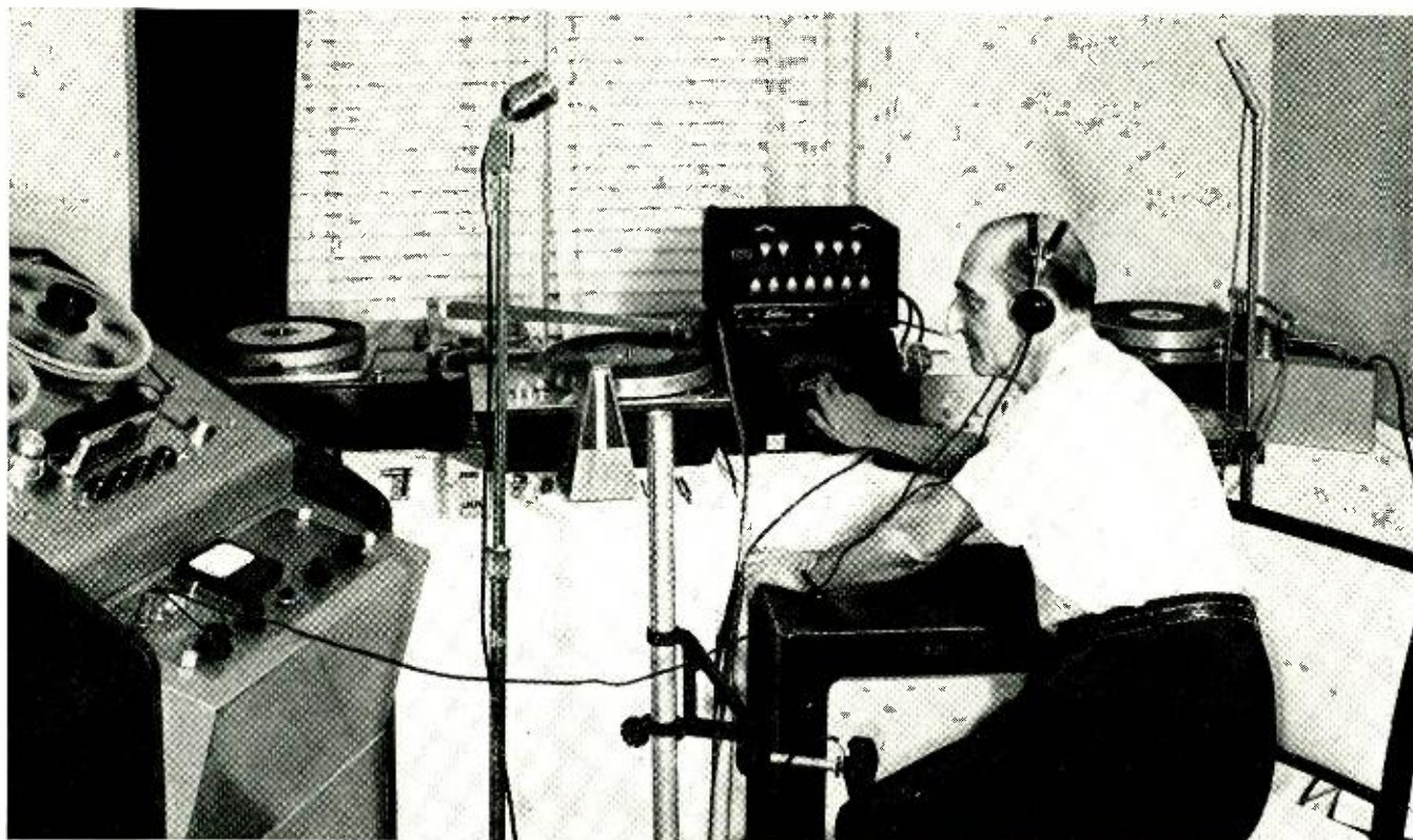
With stroboscopic frequency meter, the author checks steadiness of a 440-cycle tone recorded for reference on tape recorder.
