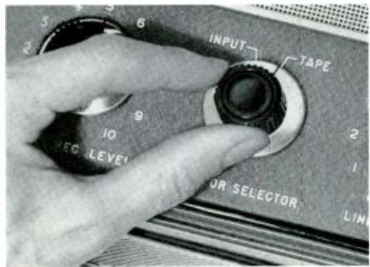
The Ampex 600 monitor selector switch lets you make an instantaneous listening comparison between what is fed to the tape and what the tape plays back to you. (Ask your local Ampex distributor for this demonstration*)
