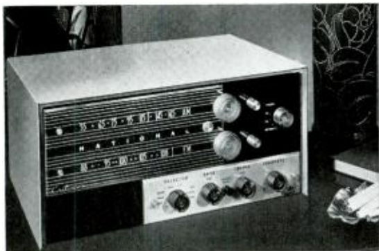
Criterion tuner has separate FM, AM sections. Preamp is in slot.
