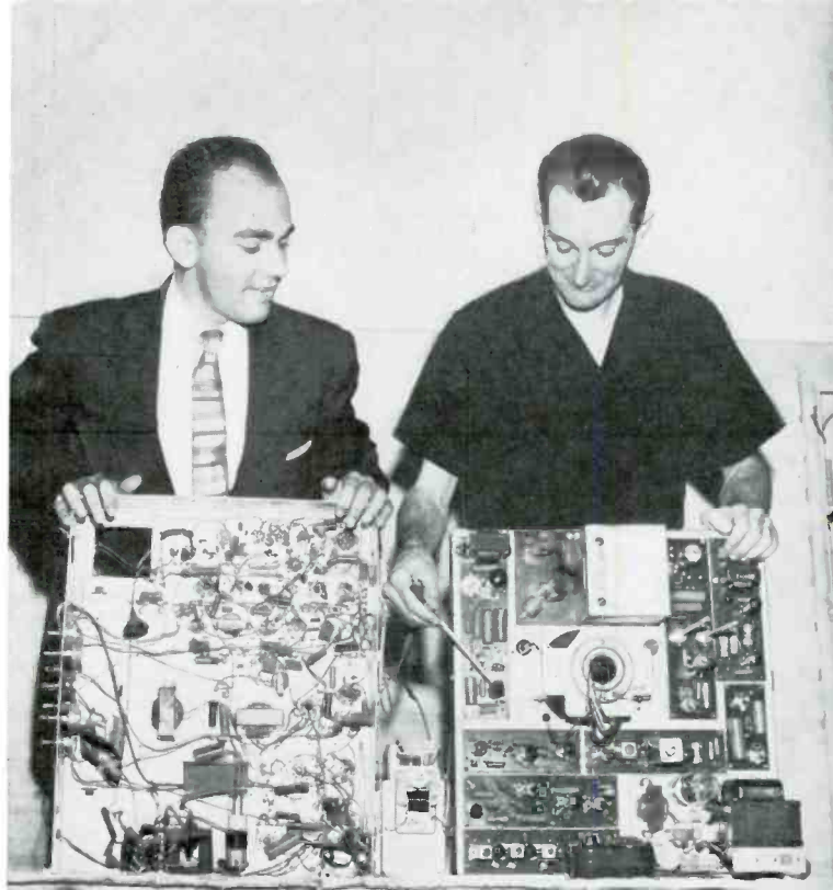
No more “jungle” of wires. Chief Engineer Fred Miller (right) makes a side-by-side comparison of a WalSCO PC-9 (right) with a conventional, complicated chassis. Bob Mueller, Walsco Sales Manager, observes simplicity of vertically mounted, printed circuit design.
