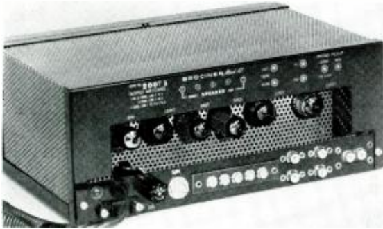
Back of Mark 12 cage carries clear indications for wiring.
