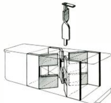
Detail shows armature and pole pieces.
