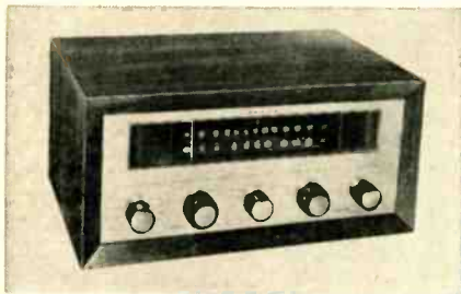
The Bogen R765 tuner has delayed AFC.
