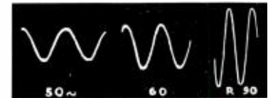
Fig. 31. Input 1 watt. Totally enclosed cabinet, 4 1/2 cu. ft. with interior loosely packed with soft absorbent material. The wave form is very good down to 50 cycles where it looks better than Fig. 24 because it was improved by indoor conditions. There is no distortion at resonance at 90 cycles.
