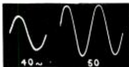
Fig. 25. Input 1 watt. Free-field. Vent output from 12-in. unit in reflex B, area 8 by 3 in. Note excellent shape at 40 cycles. At 50 cycles the output is double the frontal cone emission.
