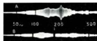
Fig. 22. Input 1 watt. A) Open back cabinet No. 7. Microphone placed at rear of cabinet in a central position: Note pronounced peak around 190 to 210 cycles. B) Cabinet No. 8. Microphone just inside as at A. Note reduced sound level and absence of peaks.
