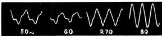
Fig. 23. Input 1 watt. 12-in. unit on 3 ft. by 2 ft. 6 in. baffle in corner of test room. It should be mentioned here that the wave shape in the region of 50 cycles was usually rather better in the test room than in the open air. Phase effects and reflections are well beyond the scope of these articles, but they obviously affect the microphone position. The live room pictures are therefore put forward as being a reasonable presentation of a varying phenomenon.
