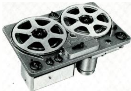
Direct-drive hysteresis motor is big feature of new model 1502.
