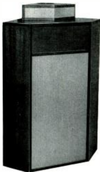
The three-speaker corner-system as originally designed, with tweeter up-ended in movable, open-sided box atop cabinet. Newer version is neater.
