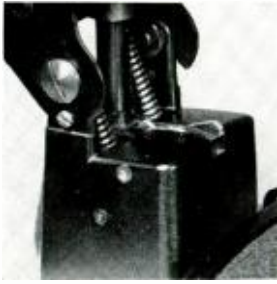
Close-up of base of over-arm mechanism on record changer shows two small feelers which control stop mechanism after last record and set-down position of arm for 10 and 12-inch records.
