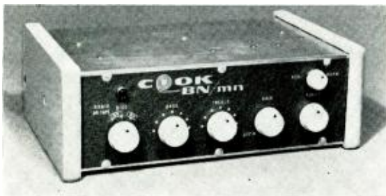
Two-channel preamp simplifies operation of binaural systems.
