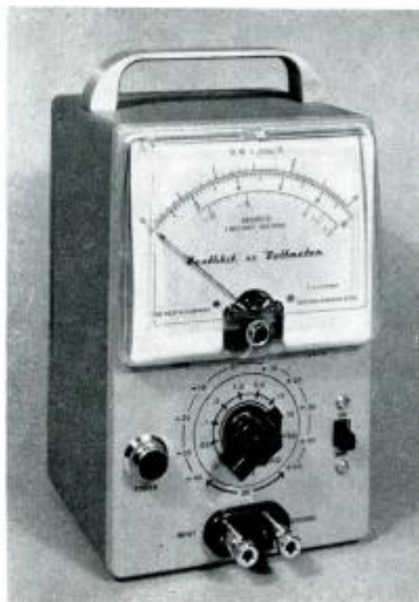
Fig. 6. The very sensitive AC voltmeter, reading to five-thousandths of a volt, in completed form.
