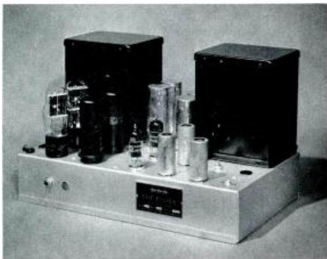
Fig. 3. Forty-watt, hi-fi amplifier provides exceptional response.
