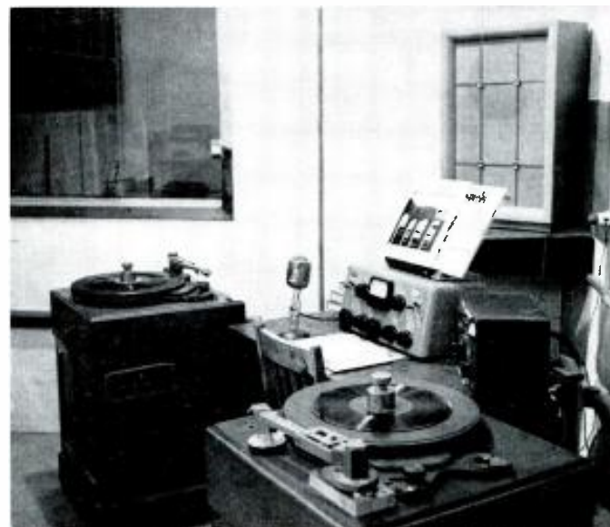
Control desk at the Woburn studios. Note the five-pound weights on the turntables: they're used to flatten warped or buckled records.
