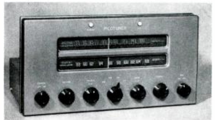
Fig. 2. AM-FM tuner includes phono preamplifier and all controls.
