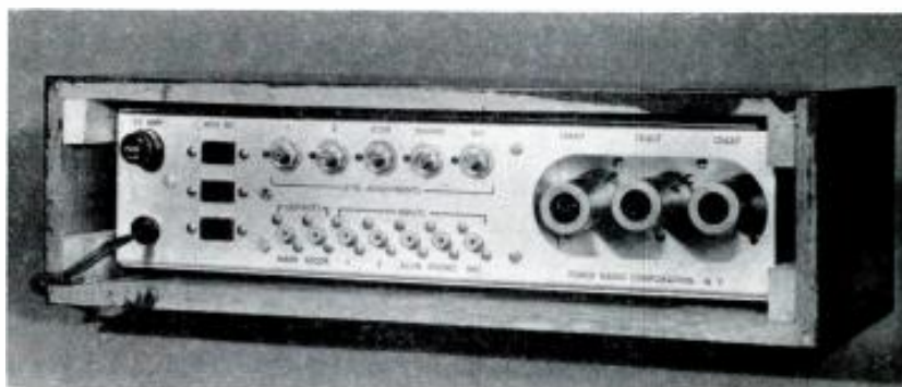
Fig. 2. Rear of chassis has five input and two output channels.
