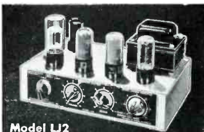
Power output, 8 watts, 16 watts peak. Distortion of 8 watts, 1% harmonic and 4% intermodulation. Frequency response, \pm 1 dB, 20 to 20,000 CPS, at 8 watt level. $36 50
