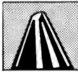
Sapphire Stylus after 30 playing hrs.
