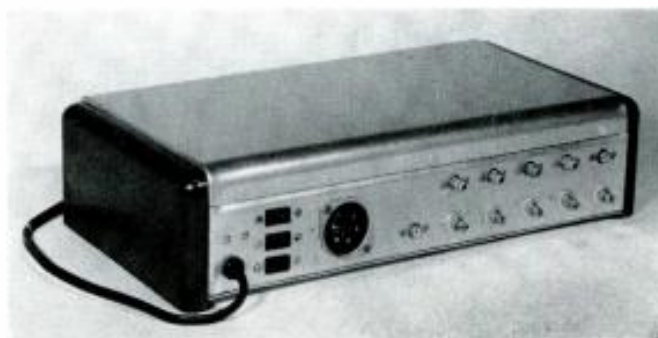
Fig. 2. Rear of preamplifier. Large socket is for power cable.
