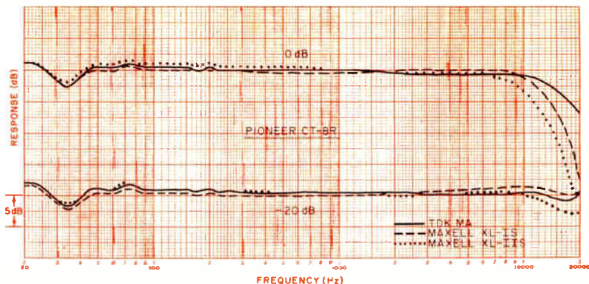
Frequency responses for three different types of tape.
