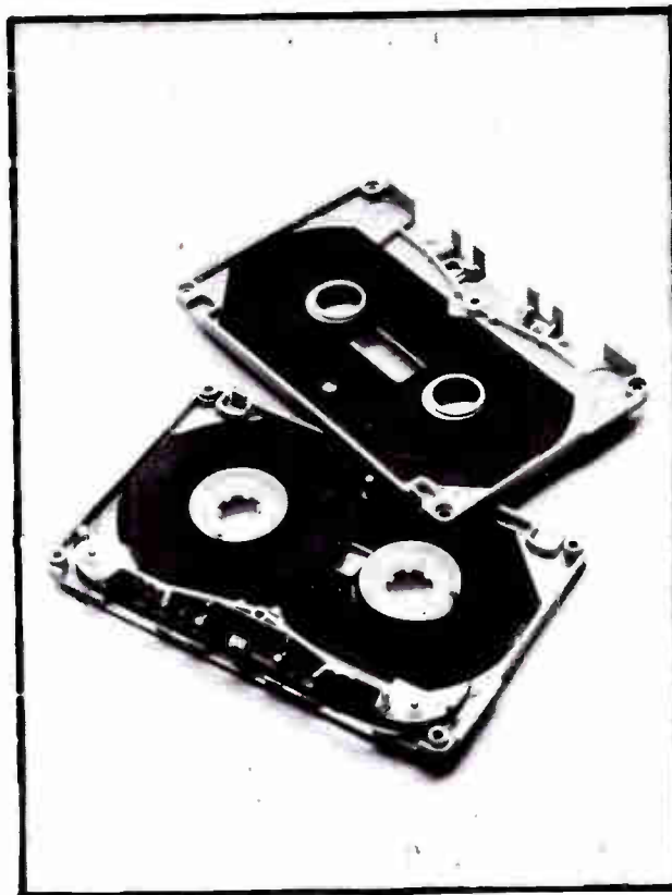
Cassettes are more like open-reel systems except two reels are housed within a plastic shell.
