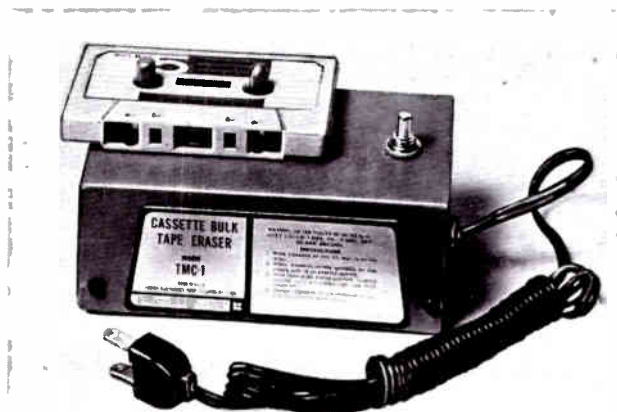
Cassette bulk tape eraser, the TMC-1 from Robins, operates from 50-60 Hz, 110-V line.
