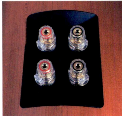
The metal strap normally connecting these two sets of speaker terminals has been removed for biwiring or biamping.
