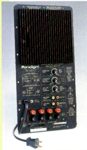
The back panel of Paradigm's PW-2200 powered sub has level, cutoff-frequency, and phase controls.
