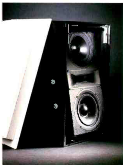
Triad's THX-certified Inwall Gold/10 LCR ($1,100 each) has two 6½-inch woofers and a 1-inch fabric dome tweeter with a dispersion lens — all mounted on a pivoting baffle.
