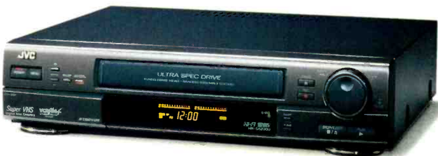
A Super VHS VCR such as JVC's HR-S5200U ($850) provides 400 lines of horizontal resolution, suitable for recording high-quality broadcasts delivered via a Digital Satellite System.
