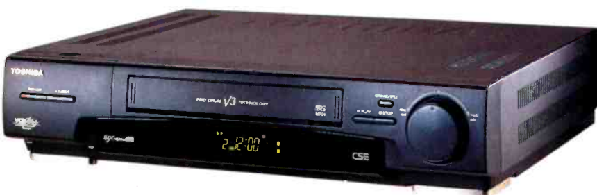
The M761 ($499) is one of three models from Toshiba that have six video heads and a flying preamp to help improve the picture quality of tapes recorded in the EP mode.
