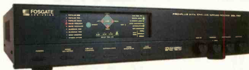
Fosgate's DSL-2 Pro-Plus (above) is representative of high-end outboard surround decoders; Denon's AVR-1010 receiver (right) incorporates Dolby Pro Logic decoding and six channels of amplification.
