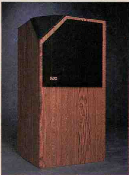
Ohm's FRS-7 uses a corner-mounted tweeter to generate a controlled-directivity sound field. Its 6½-inch woofer is acoustically coupled to a 10-inch passive radiator for extended bass response. Price: $680 a pair.
