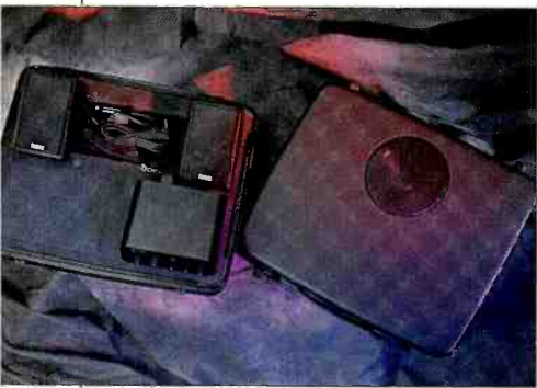
The BassCase has cutouts in its damping foam to hold the satellite speakers, the amplifier, a portable CD or tape player, and the connecting wires.
