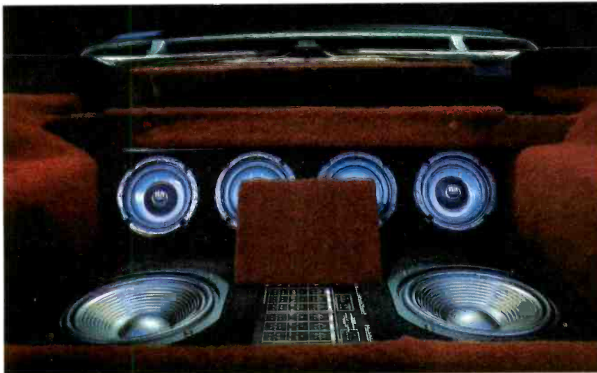
The Corvette's imposing dash has a "rack" of Eclipse gear. Custom door work (top) accommodates Nakamichi speakers, and part of the car's electrical system was modified (middle). Five Rockford Fosgate amps restle in the trunk along with a custom fusebox and the rear speakers. At left, the finished trunk layout, with the M&M mid-bass drivers, Nakamichi subwoofers, and Alpine 3401 parametric equalizer.
