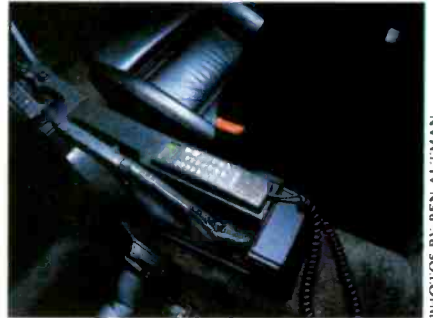
The Alpine 7390 cassette receiver and CD controller unit looks natural in the BMW's dash. Two 15-inch Pyle subwoofers are hidden inside the back seat (top), and each front door has a midrange and tweeter in a custom Z-Box enclosure (middle). There's even room for a Mitsubishi Mesa 95 cellular phone. The trunk holds the Pyle power amplifiers that make this system scream.
