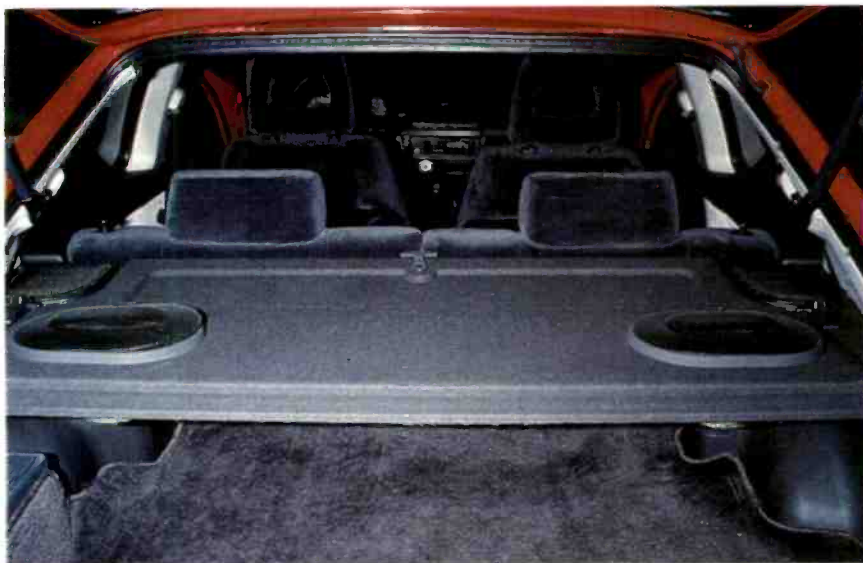
The Acura's dash holds a Sony XR-7200 cassette tuner, the trunk (top) a side-mounted Sony CDX-A20 ten-disc CD changer. The rear deck sports 6 x 9-inch Pioneer TS-6966 triaxials, and two Sony XM-701 amplifiers are mounted forward of the spare tire. At left, a look at the removable rear deck.
