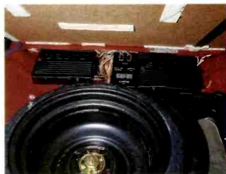
The Acura's dash holds a Sony XR-7200 cassette tuner, the trunk (top) a side-mounted Sony CDX-A20 ten-disc CD changer. The rear deck sports 6 x 9-inch Pioneer TS-6966 triaxials, and two Sony XM-701 amplifiers are mounted forward of the spare tire. At left, a look at the removable rear deck.
