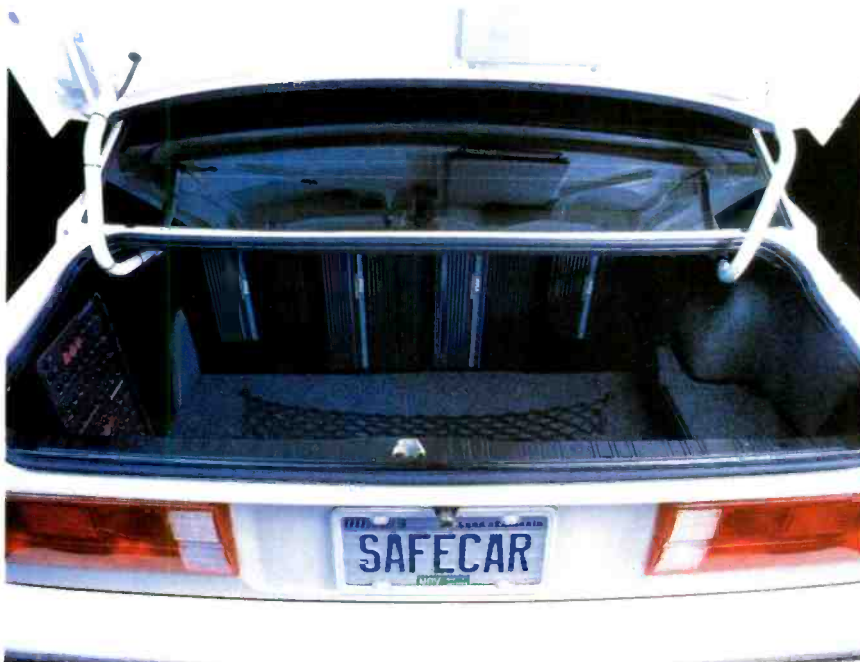
The Alpine 7390 cassette receiver and CD controller unit looks natural in the BMW's dash. Two 15-inch Pyle subwoofers are hidden inside the back seat (top), and each front door has a midrange and tweeter in a custom Z-Box enclosure (middle). There's even room for a Mitsubishi Mesa 95 cellular phone. The trunk holds the Pyle power amplifiers that make this system scream.
