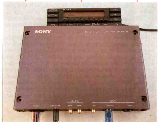
Sony's CDX-2001 DiscJockey CD changer ($1,400) is the first car player to use eight-times oversampling. Its ten-disc magazine is interchangeable with those of other Sony home and
