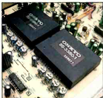
Dual Acculinear D/A Converters with calibrated accuracy to the 4th Significant Bit.
