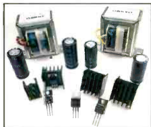
Dual transformers in the DX-7500 thoroughly isolate digital and analog stages.
