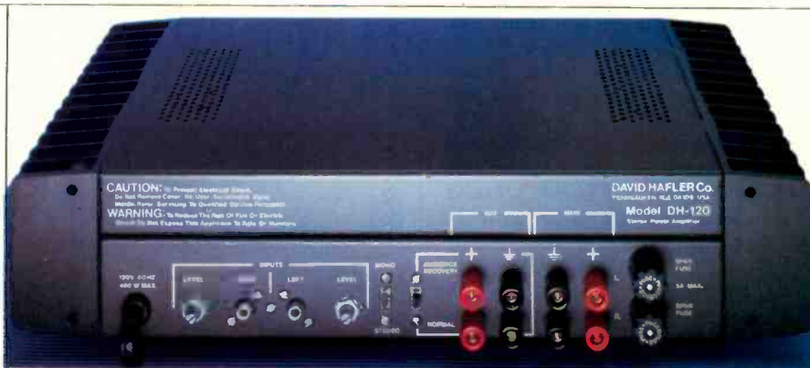
The Hafler DH-120 has extra binding-post terminals to drive ambience speakers.
