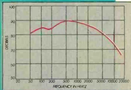
Figure 2 (below). The average energy distribution of rock music. Classical music has a lower peak frequency and rolls off slightly faster.
