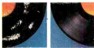
(Left) Styrofoam beads are attracted to static charge left on record after cleaning with Discwasher D3 ®
