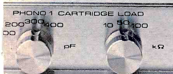
Impedance switches that let you get the most out of your cartridge.
