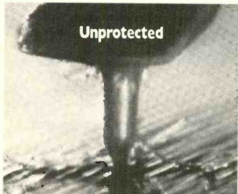
Magnification shows the record vinyl wearing away.
