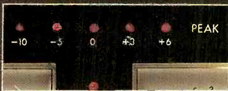
5 LED peak level indicators help eliminate distortion.
