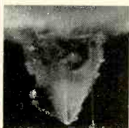
Accumulated grit on stylus that looks "clean" to the naked eye.
