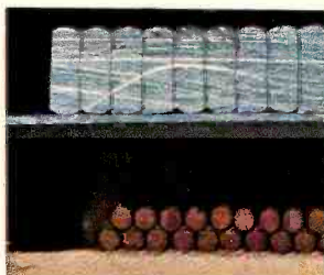
The voice coil consists of flat aluminum conductor wire wound on-edge on an aluminum core, eliminating the inefficient air gaps between the round copper windings of a conventional voice coil.
